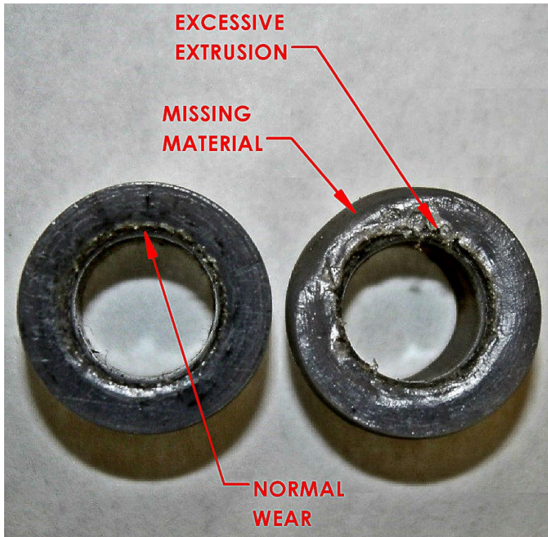
Figure 13 Dynamic Seal Inspection
